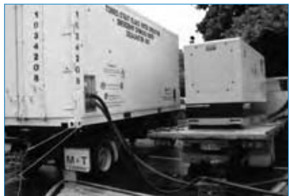
A Mobile Desalination Unit ready for use.
