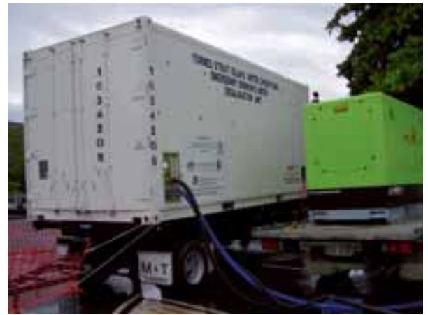
A mobile desalination unit on standby for emergency water production
