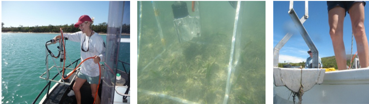
Figure 1. Subtidal mapping of seagrass meadows using CCTV system and van Veen sediment grab.
