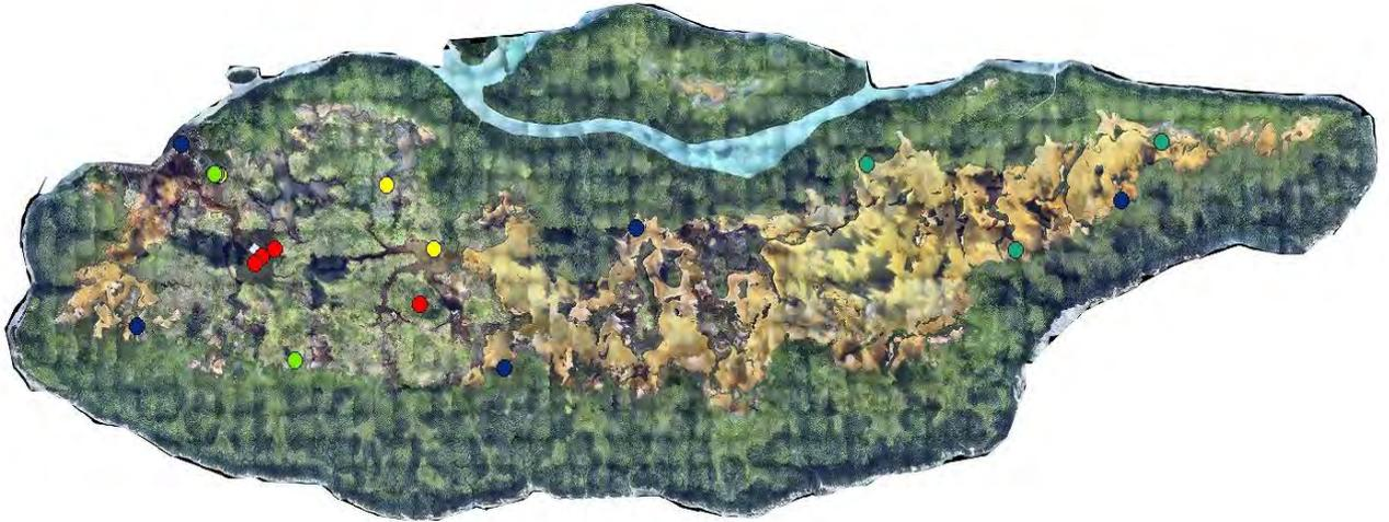
**Figure 4.7** Conductivity (salinity) measured on Badu Island. Red (<2mS/cm), yellow (2-12mS/cm), light green (12-34mS/cm), dark green (34-44mS/cm), and dark blue (44-66mS/cm)
