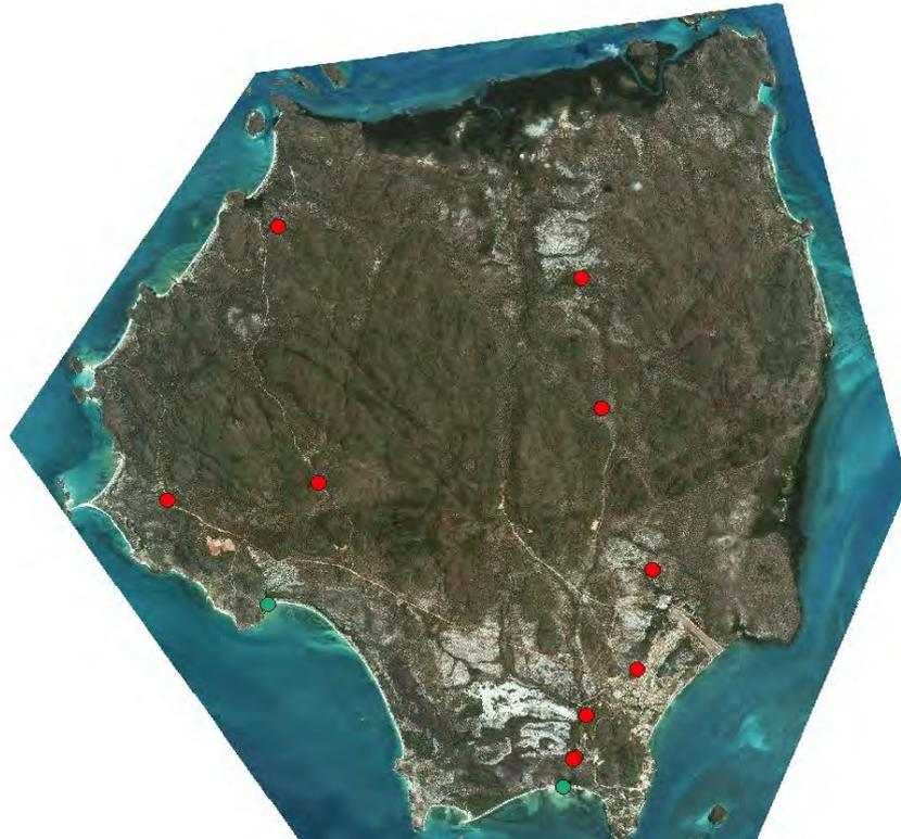
**Figure 4.8** Conductivity (salinity) measured on Mabuiag Island. Red (<2mS/cm), yellow (2-12mS/cm), light green (12-34mS/cm), dark green (34-44mS/cm), and dark blue (44-66mS/cm)
