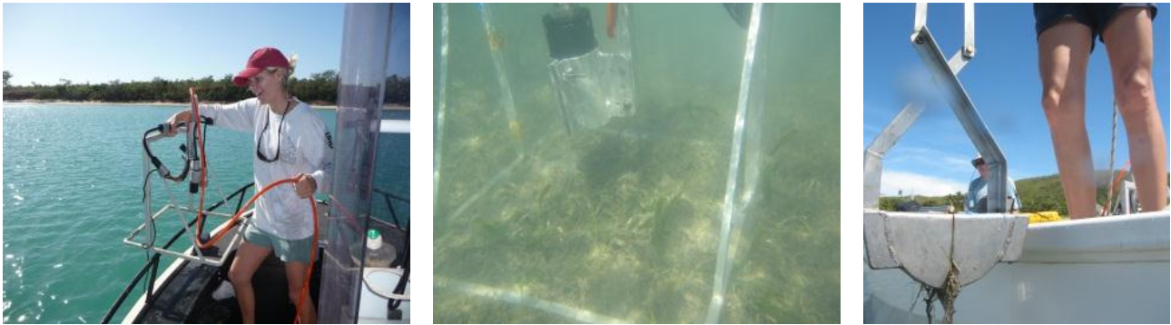
Figure 3. Shallow subtidal mapping of seagrass meadows using CCTV system and van Veen sediment grab.
