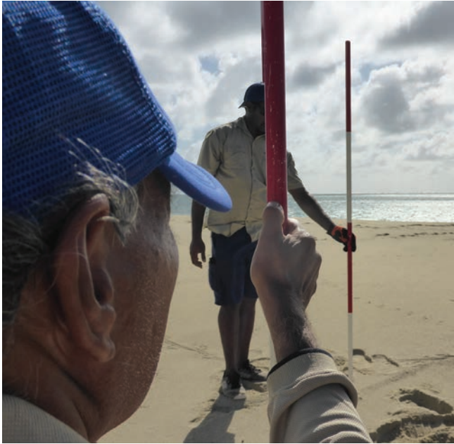
Ranger Joseph Dorante measuring changes to beach (beach profiling)
